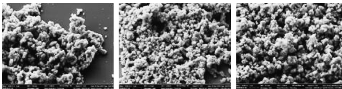
Fig. 1. SEM images of the (a) original Hombikat TiO 2 ; (b) calcined Hombikat TiO 2 ; (c) Hombikat TiO 2 with 5% ZnO loading.
